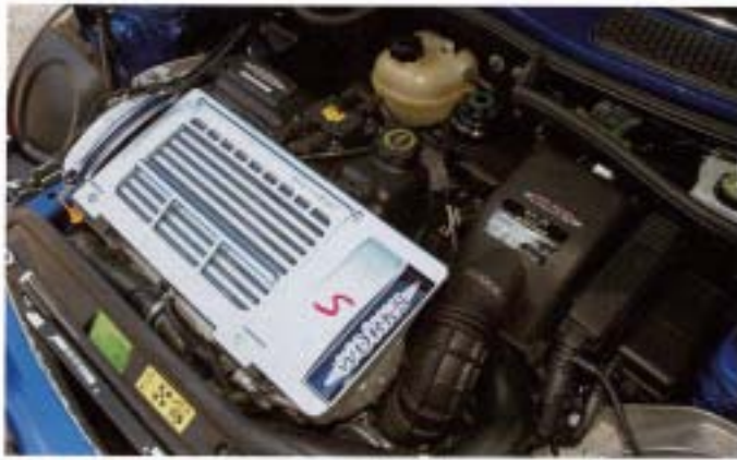
The John Cooper Works Mini Cooper S has been a good option choice ever since MINI started installing the upgrades as factory options. The added power is achieved by replacing the cold air intake system, head, supercharger, and exhaust, and reprogramming the ECU. The factory option package also includes JCW brakes and limited slip differential.
